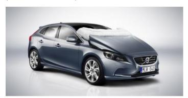
In a collision with a pedestrian or cyclist the bonnet lifts up, an airbag is deployed and the impact on the pedestrian is mitigated.
